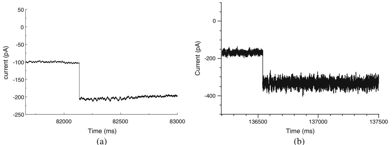
**Fig. 7** Current trace of phi29 connector protein molecule inserted into a microfluidic lipid-bilayer in (a) 500 mM NaCl buffer solution and (b) 1 M NaCl buffer solution
