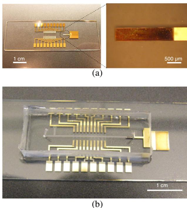
**Fig. 3** Picture of the fabricated device. (a) patterned electrodes on glass substrate (right) and Ag/AgCl electrodes at the end of gold electrodes (left), and (b) attached PDMS microchannel
