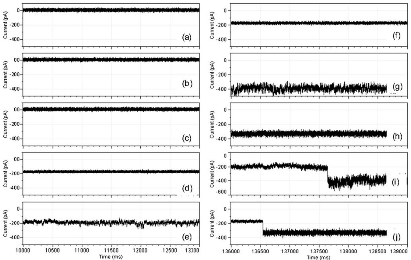
**Fig. 6** Current traces from 10 lipid bilayers with different numbers of the inserted phi 29 nanopore. (a–c) 0 inserted nanopore, (d–f) 1 inserted nanopore, (g–h) 2 inserted nanopores, and (i and j) current trace during the phi 29 nanopore insertion
