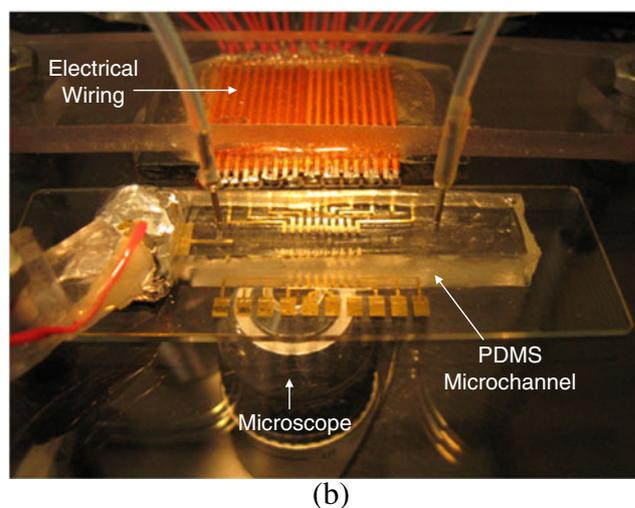
**Fig. 4** Picture of the microfluidics showing the experimental set-up. **(a)** The system inside EM shielding cage. **(b)** Electrical connection to each electrode on the microscope for visualizing the formation of lipid bilayer with electrical monitoring
