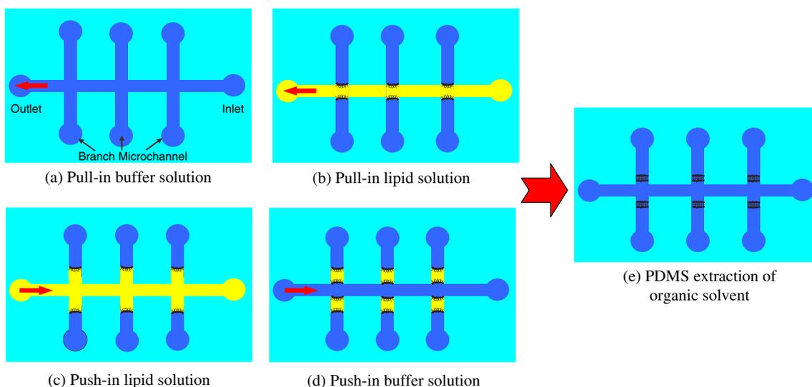
**Fig. 1** Schematic illustration of push-pull junction capturing for a formation of multiple lipid bilayers inside an array of microchannel
