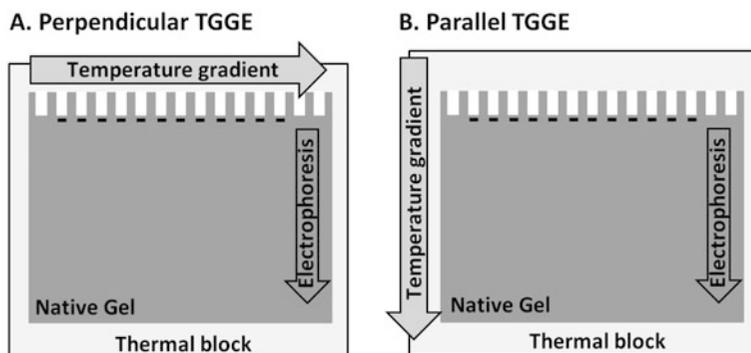
**Fig. 1** Demonstration of (a) perpendicular and (b) parallel settings of temperature gradient gel electrophoresis
