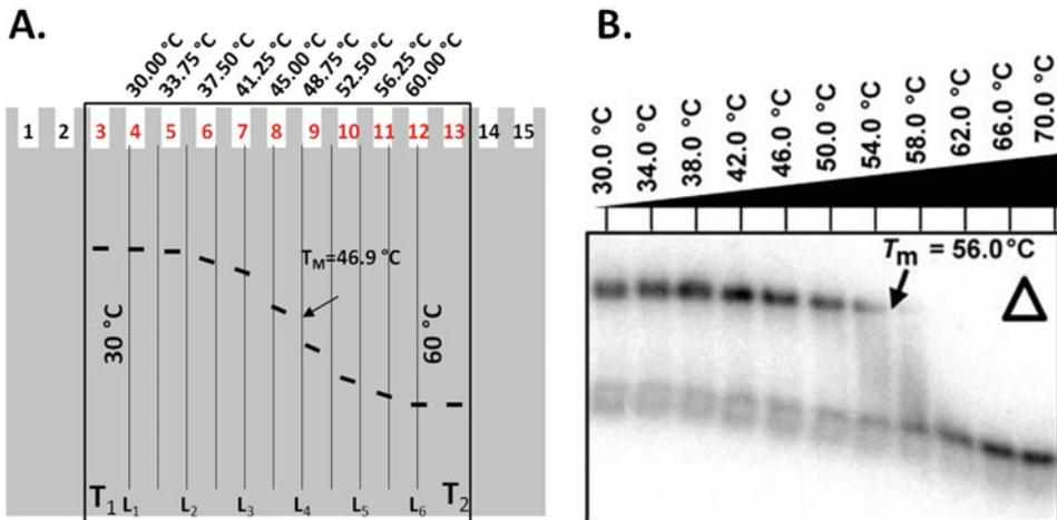
**Fig. 4** Example of RNA complex melting point determination. (a) Calculation of temperature on each PAA well based on known the temperatures of L1–L6. (b) Melting temperature of P-32 labeled RNA triangle NP determined using TGGE system. (Image obtained from ref. [15] with permission from NAR, Oxford University Press)
