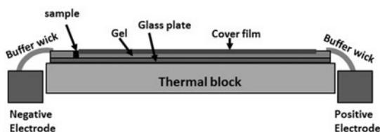
**Fig. 2** A detailed view of customized TGGE system. (a) Photograph of complete assembly unit. Schematic top and side views with descriptions of components are shown in panels **b** and **c**, respectively
